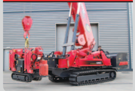
Outriggers stowed to traverse a narrow opening
