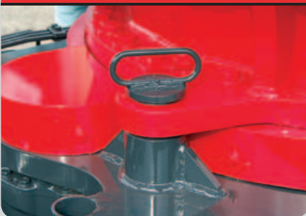
Safety pin and micro-switch keeps boom fixed in position
